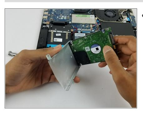
Remove the hard drive from the mounting bracket.
