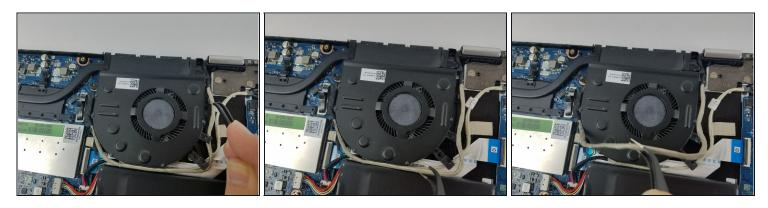
• Using the Precision Tweezers, remove the 2 gray wires around the fan from their clips.
