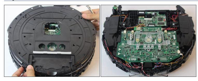
• Lift the top plate slowly, being careful not to damage the vacuum components while exposing the motherboard.
