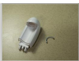
Using Needle Nose pliers remove metal roller track on both sides of the Tweezers Head.
