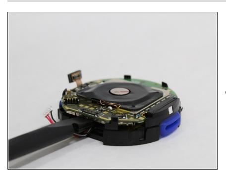
The battery is secured to the back of the motherboard utilizing a sticky pad. Gently separate the battery from the board while making sure
