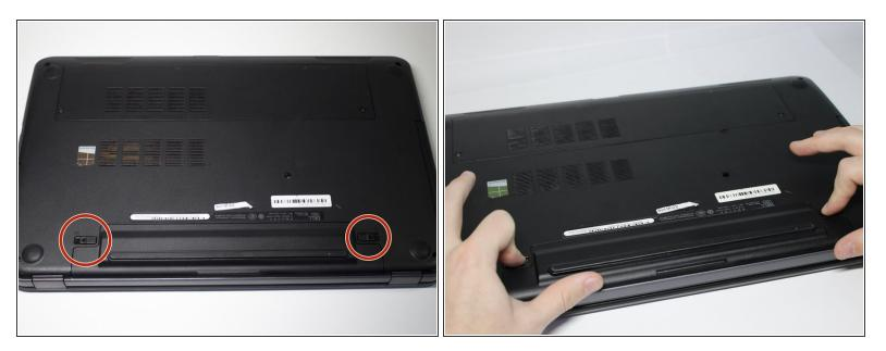
Slide each latch away from the battery to unlock it.
