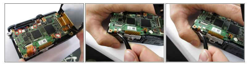
• Using tweezers, pull out the shown connectors
