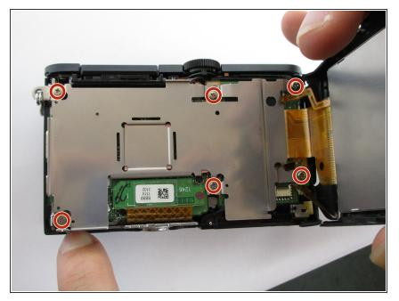
Lift up the screen, and use a Phillips #000 screwdriver to remove the (6) six screws holding down the underlying metal plate.
