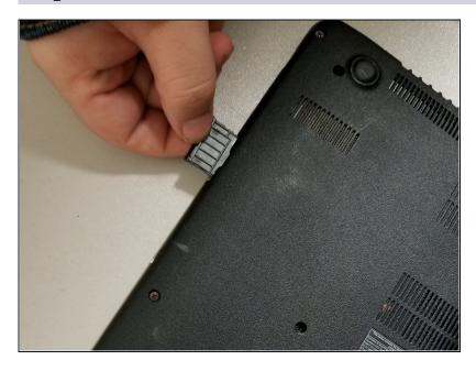
Remove the storage tray on the left edge of the device.
