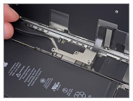
• Remove the lower display cable bracket.
