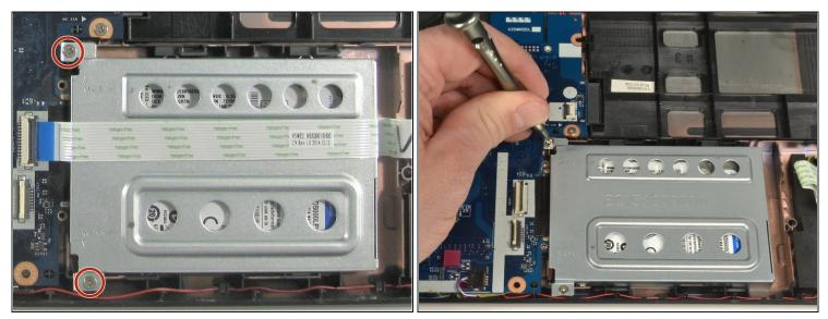
• Use a #0 Phillips screwdriver to remove the two 4mm screws securing the hard drive carriage in place.
