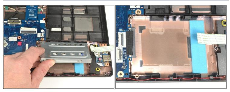
• Lift up the hard drive carriage on the edge closest to your body to remove it.
