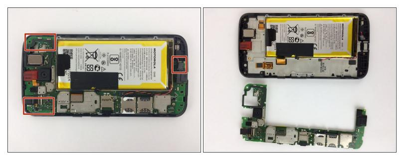
• Using the tweezers pull up on the three corners of the motherboard until it comes out.
