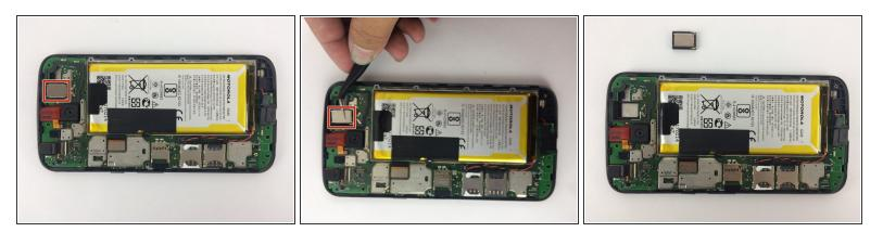
Using the tweezers, slide them under the speaker and pull the speaker out.
