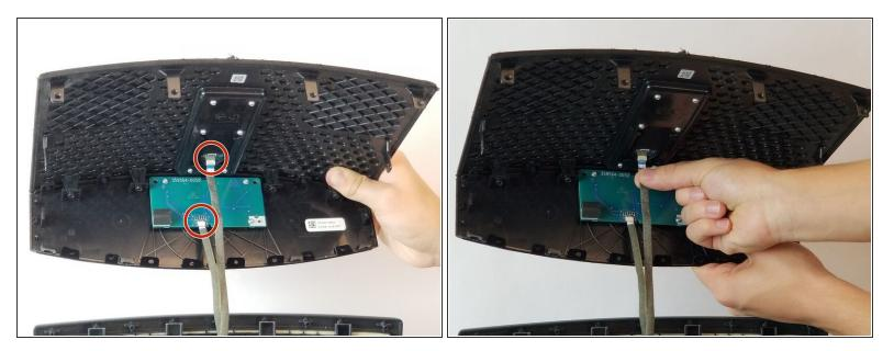
After lifting the cover, you will see two ribbons attaching the cover to the speaker. Gently remove these ribbons by pulling straight down.
