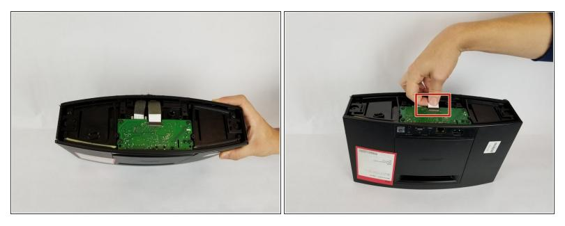
• Gently pull the white ribbon from the connector on the top side of the motherboard.
