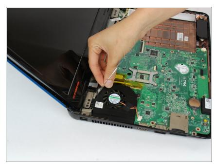
• Remove the fan from the device.
