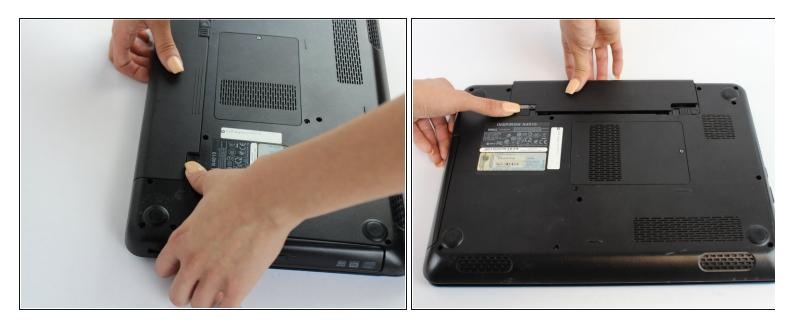
• While holding the left-hand switch to the left position, pull the battery away from the laptop.
