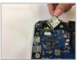
• Lift up the network card and remove it from the motherboard connector.
