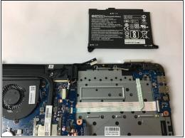
Carefully disconnect the cable connecting the top of the battery and remove the battery.
