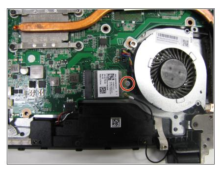
Using the <u>Phillips #00 screwdriver</u>, remove one 0.5 mm screw.
