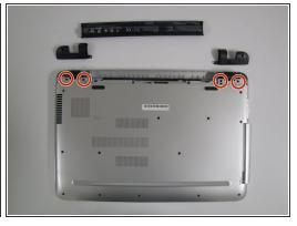
Remove the black corner covers on either side of the battery to reveal four additional 6.5mm
