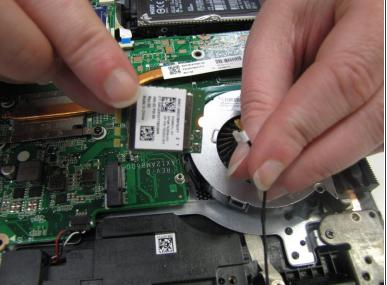
After unscrewing the screws, lift the Video Card up from the motherboard. Disconnect the wire from the Video Card by gently wiggling the gold end on the left corner of the card.
