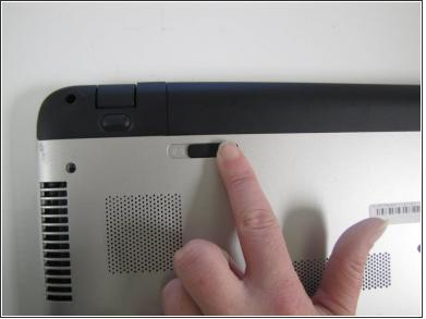
In the upper left hand corner, slide the bar with the lock icon to the right. This will unlock the battery.
