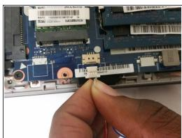
• Using your fingers, remove the speaker connector from its port by sliding it out.
