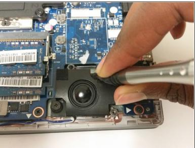
Remove the two 8mm Phillips #1 screws holding the right speaker in place.
