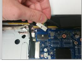
Using your fingers, unplug the battery from the laptop by taking the plug out of its socket.
