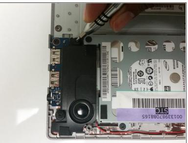
Remove the two 8mm Phillips #1 screws holding the left speaker in place.
