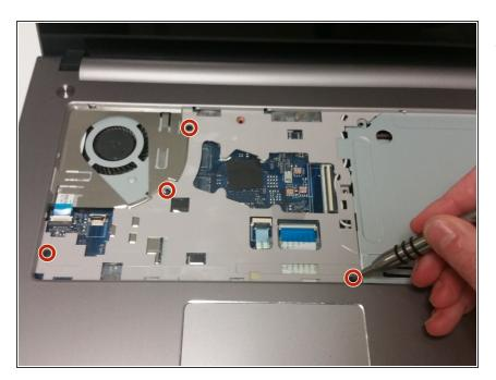
Remove four 7mm Phillips #1 interior screws.
