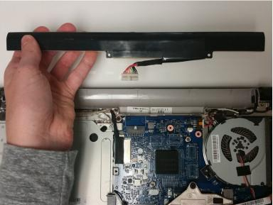
Using your hand, remove the battery from the laptop by lifting one side and then pulling it out of its slot.
