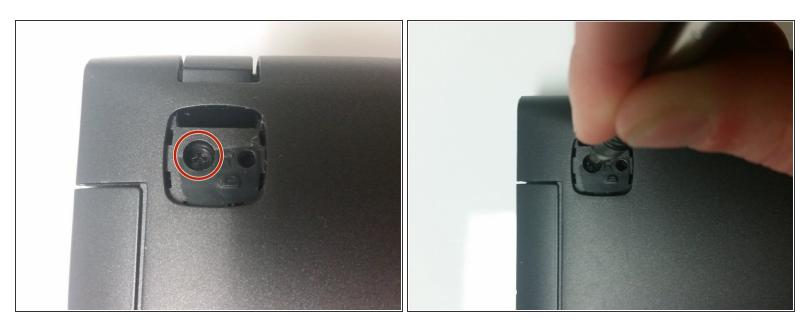
Remove the 7mm Phillips #1 screw beneath where the foot was. Do this for both sides.
