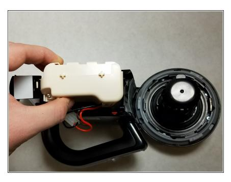
Remove the battery unit by pulling it out of the main body.
