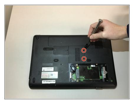
Unscrew and remove the two 5mm
