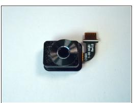
Remove the optical joystick.
