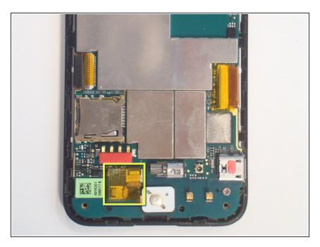
Remove the tape covering the optical joystick ribbon cable.
