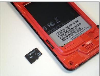
Pull the MicroSD card straight out of its slot.
