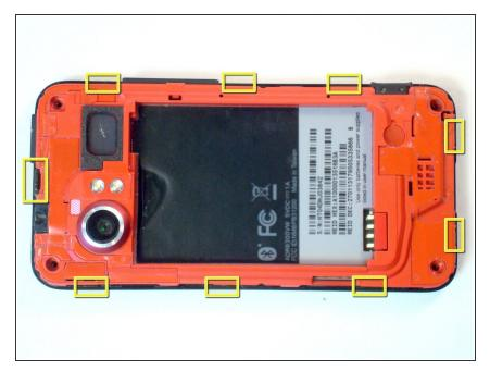
The rear inner frame is attached to the front case by nine plastic clips, marked here for reference.
