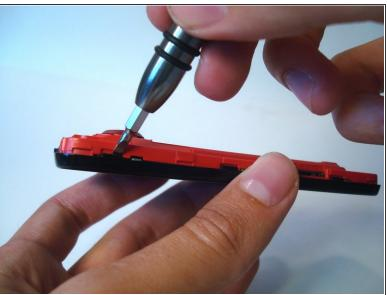
Loosen the clips on the side next to the camera using the method described in the previous step.
