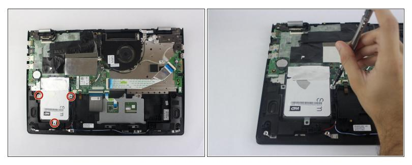
• Using the Phillips #0 screwdriver, remove the (3) three 3 mm screws.
