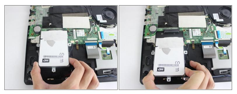
• Carefully, using your hand, remove the hard drive from the laptop.
