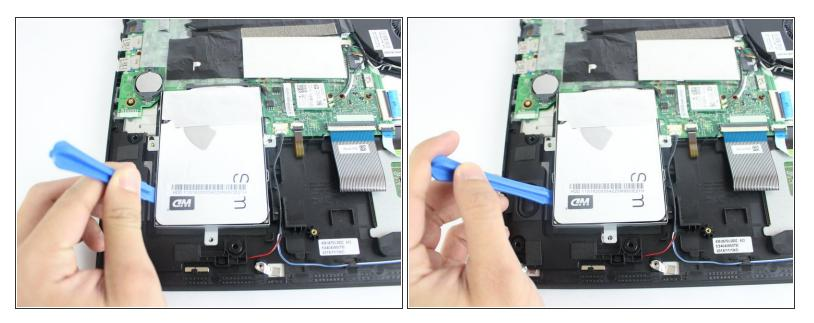
Slide the drive away from the connector by applying pressure on the two side tabs where screws were removed. Use a plastic opening tool as a lever to lift the drive out.
