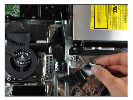
De-route the optical drive data cable out of the rear case.
