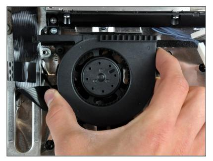
Lift the optical drive fan up off the plastic posts protruding from the rear case.
