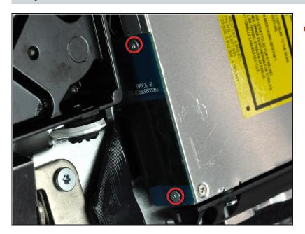
Remove the two 3.5 mm T6 Torx screws securing the optical drive connector to the optical drive.
