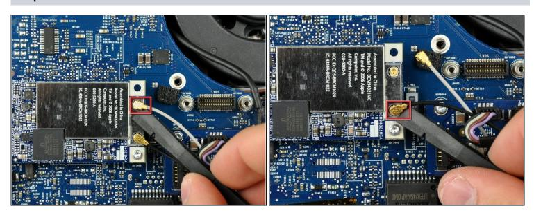
Use the flat end of a spudger to pry both AirPort antenna connectors up off the AirPort card.
