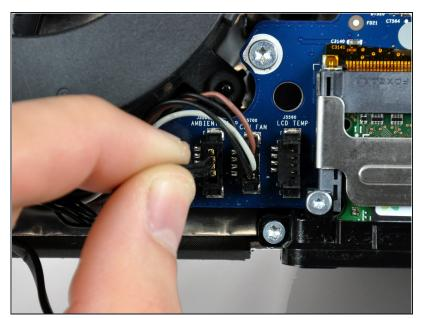
Disconnect the ambient temperature sensor cable by pulling its connector straight up off the logic board.
