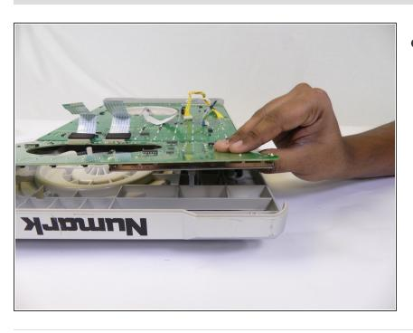
Carefully remove the circuit board from its housing.
