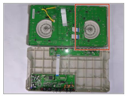
Locate the top right PCB circuit board.
