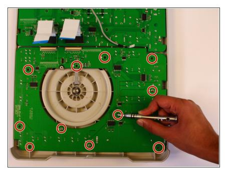
Loosen and remove the 11 12mm screws from the circuit board using a Phillips #2 screwdriver.
