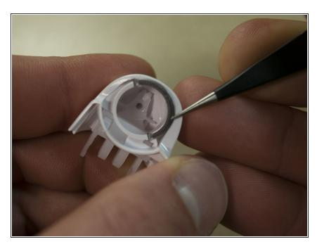
Replace Metal Roller Tracks on both sides of the Tweezer Head.
