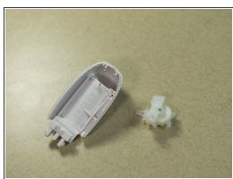
Use a spudger to pry the gear housing unit from the base.
