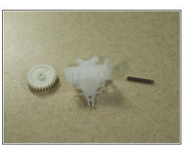
• Use your thumbnail and a pair of needle nose pliers to push out the gear housing retention pin.
