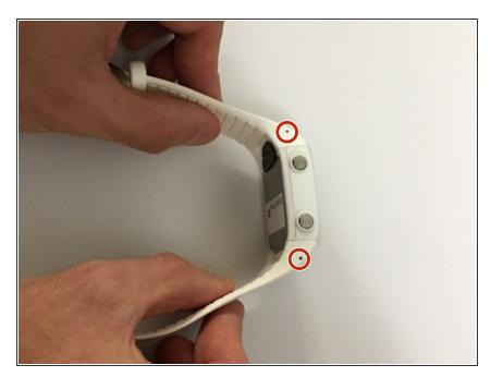
Insert a standard paper clip into the holes on both sides of the watch that connect the watch's face with the wrist strap.
