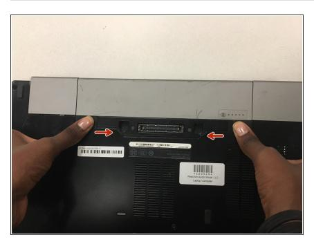
Unlock the two latches on the back by sliding them inwards.
