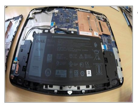
Remove the battery from the motherboard extension connector
