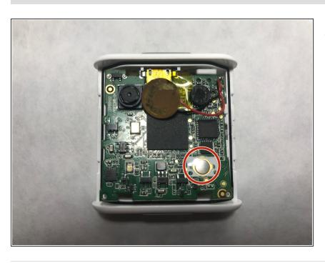
Replace capture button with advanced soldering and circuitry (circled in red).
