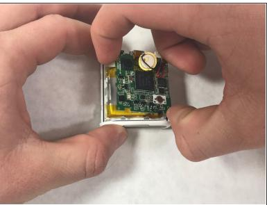
Remove the motherboard by pulling it from the edges as circled.
