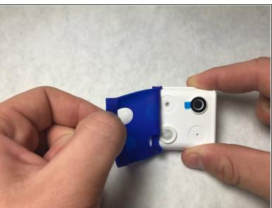
Remove any external skins placed on the device. To do so, simply lift up and peel to remove.
