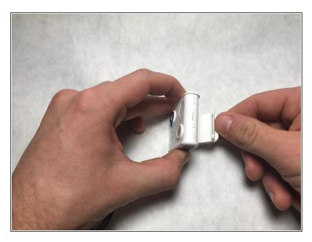
Firmly pull on the back clip in order to remove.
