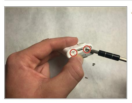
Use a Phillips head screwdriver to remove the four 4mm PH00 screws located on the sides of the device.
