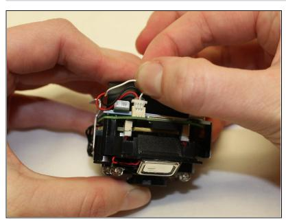
• Carefully unplug the battery from the rest of the lens.
