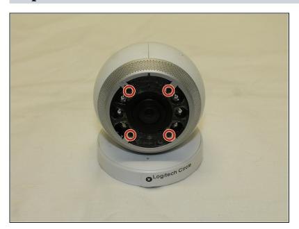
Remove the four 3mm Phillips #0 screws that hold down the first ring.
