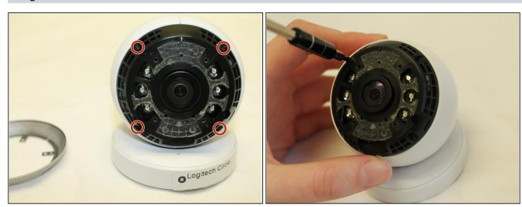
Remove the four 3mm Phillips #0 screws that hold down the second ring.
