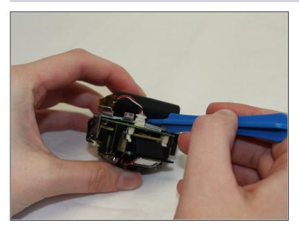
Remove the battery using a plastic opening tool. The battery is attached with sticky tape and will remove with gentle prying motions.
