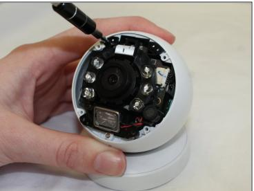
• Remove the four 3mm Phillips #0 screws that hold down the final ring. Do not remove the lens/battery bundle yet.
