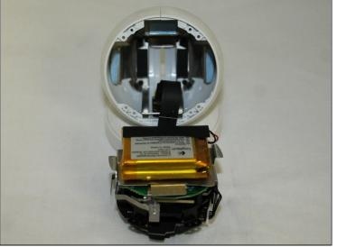
• Gently remove the lens/battery bundle from the base of the circle, being mindful of the ribbon cable.
