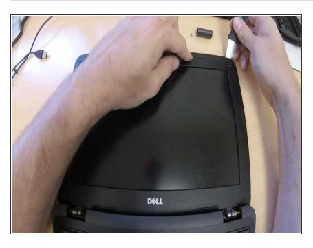
Use a plastic pry tool or blade and start in the top left corner or first left plastic ridge.
