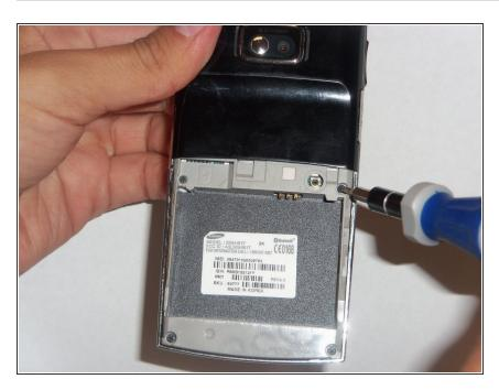
Unscrew the two screws just above where the battery was.
