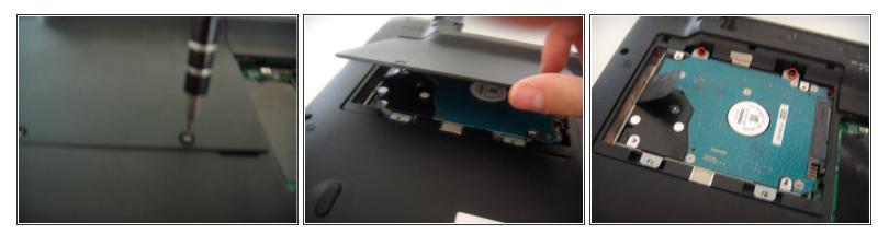
• by unscrewing these 2 star screws size 6 we can lift the hard disk plate.
