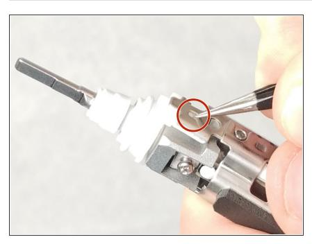
Use fine tip tweezers to push the white plastic tabs in to release the head from the innards.
