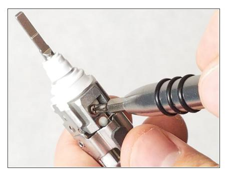
Use a Phillips screwdriver to remove the screw at the base of the metal head.
