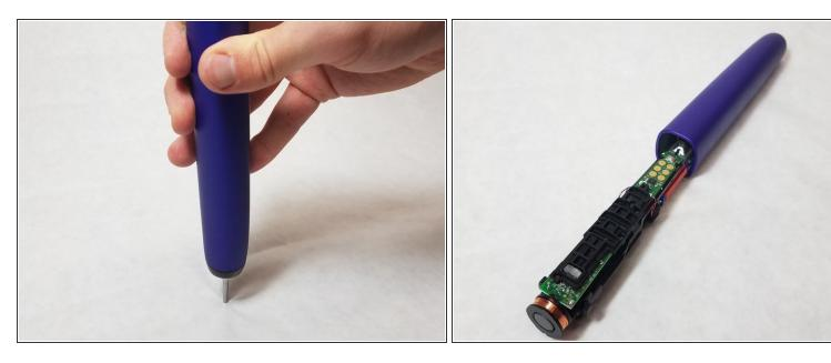
Put the metal head on a solid surface with handle perpendicular to the surface. Firmly, yet gently, push down until the internals start to slide out.
