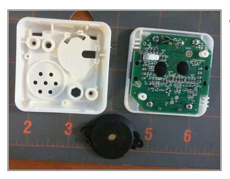
Two screws and a clip held the two halves of the case together, with two more keeping the speaker in place. Also, it looks like the only screws used in this device are Phillips! Great!
