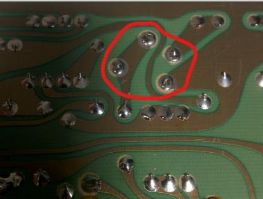
Remove the input jack by desoldering the pins on the other side of the board, you may want to use a solder remover tool to make it easier.
