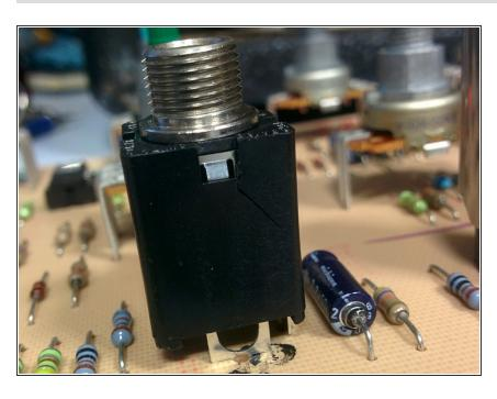
Solder the new jack in place, the jack i used had an extra pin but was not needed. i ended up bending it out of the way and it all still works.
