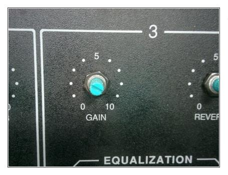
Once the jack or jacks have been replaced simply re-assemble by working backwards, remember that the dials each have a screw and a topper. when putting the toppers back on make sure the dials are turned to the minimum value and line them up to avoid confusion when being used.
