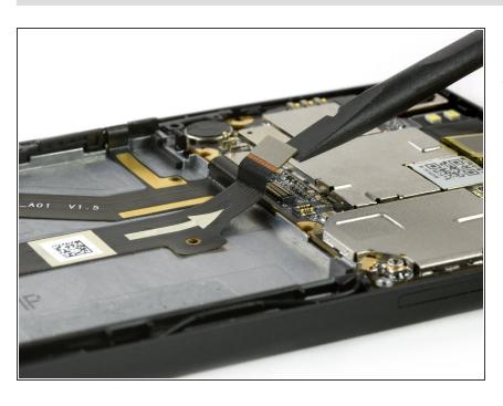
Use the flat end of a spudger to disconnect the displays flex cable from the mainboard.
