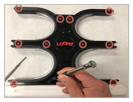
Remove the thirteen 12.7mm screws with a #1 Phillips screwdriver.
