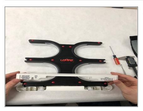
Remove the white cover. Be sure to remove the front and the back.
