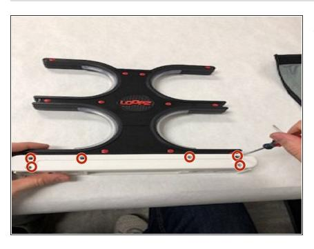
Remove the six 16mm screws with a #1 Phillips screwdriver.
