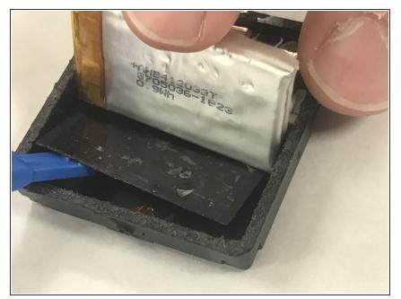
Push the black piece down while very carefully pulling the battery off.
