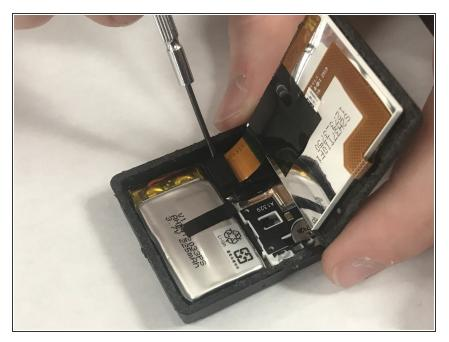
Use a plastic opening tool or spudger to lift the screen assembly press-fit connector free.
