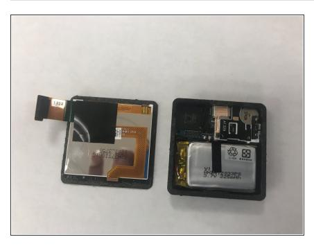
• Set aside the detached LCD screen to access the battery.
