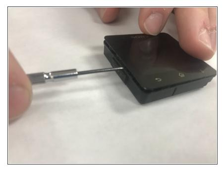
Use a plastic opening tool to carefully pry the LCD screen from the watch housing.
