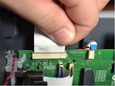
Grab the base of the white ribbon cable connecting the cover to the base of the printer and pull it out.
