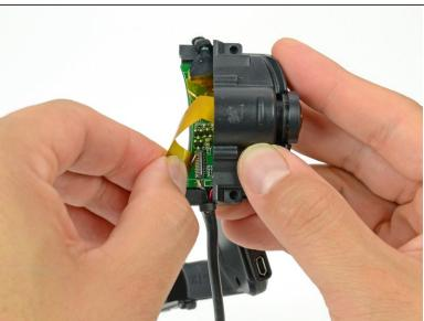
Pull the camera sensor ribbon cable straight out of its connector on the motherboard.
