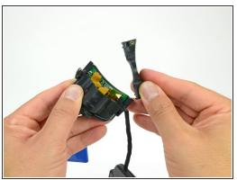
Lift the back cover off the camera housing and remove it.
