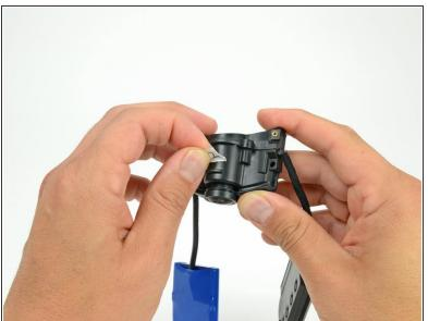
Peel the white sticker off the bottom of the camera housing.
