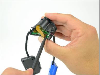
• Use the tip of a spudger to pry up the retaining flap of the camera sensor cable ZIF connector on the motherboard.
