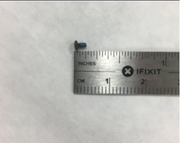
• Use the T5 Torx Screwdriver to remove the six screws that hold the back of the frame in place.
