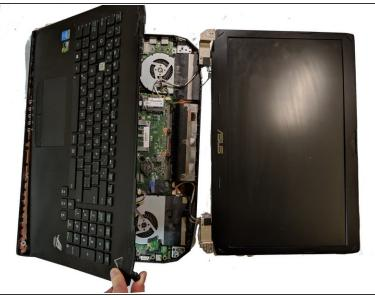
Use a metal separator to carefully separate the bottom half of the laptop.
