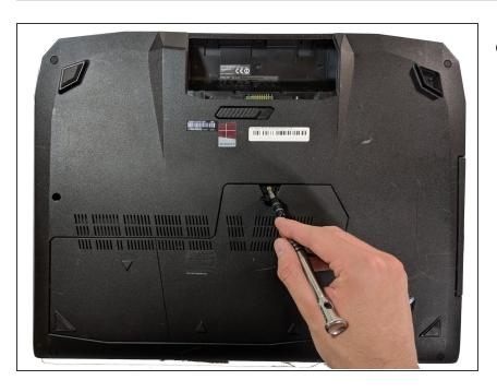
Unscrew the 5.2mm screw underneath the flap.
