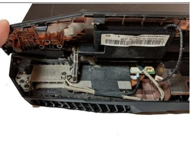
Remove the connector connecting the screen and the motherboard
