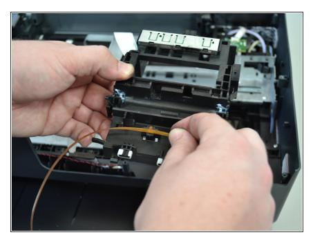
Remove the carriage belt by holding the carriage in one hand and pulling the carriage belt up with the other. To reassemble your device, follow these instructions in reverse order.
