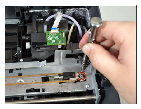
On the right side of the printer, remove the screw (6mm T9) holding the carriage belt wheel by turning the screwdriver counterclockwise.
