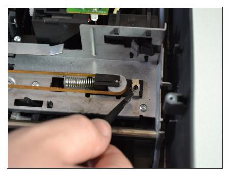
Using the tweezers, remove the metal clamp directly under the screw that was just removed by pulling up.
