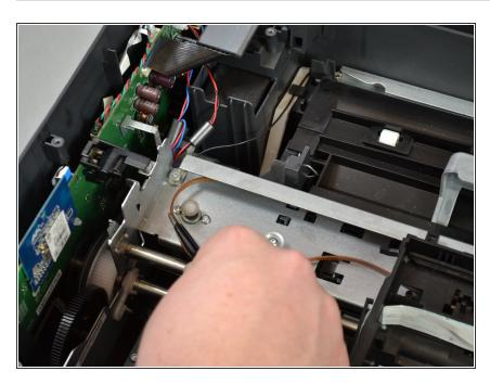
Unwrap the carriage belt from the hook on the other side of the printer using the tweezers by pulling to the left and up.
