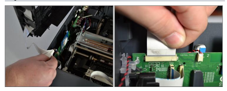
Grab the base of the white ribbon cable connecting the cover to the base of the printer and pull it out.
