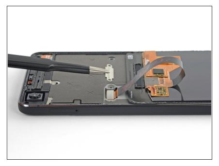
• Remove the display cable bracket.
