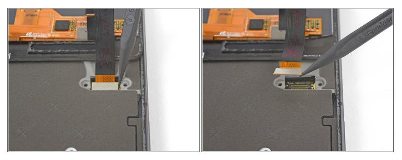
Use the point of a spudger to lift the display cable connector up and out of its socket on the motherboard.
