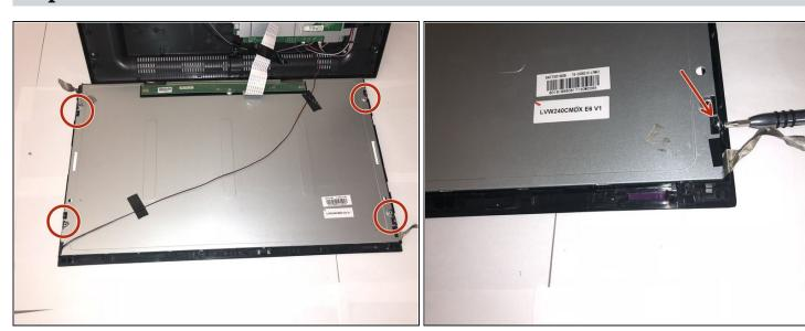
• Using the Phillips 00 Screwdriver, remove the screws that are also holding the silver rectangular piece to the house.
