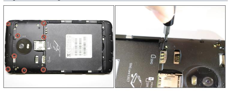
• Remove the eight (8) 4mm screws with a Phillips screwdriver.
