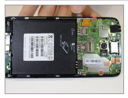
Remove the two 4mm screws shown in the picture using a Phillips #00 screwdriver.
