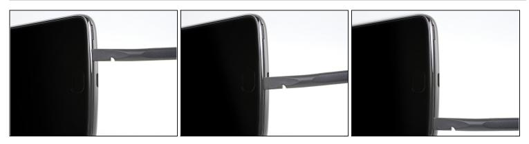
• Insert the flat end of a spudger into the seam and slide it along the bottom edge to release the clips holding the back cover to the phone.
