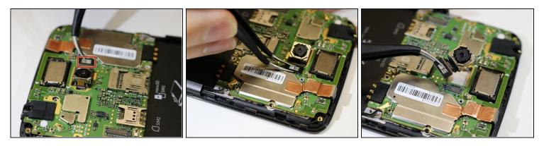
• Disconnect the marked connector with a pair of <u>tweezers</u> and remove the camera piece.
