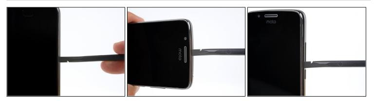
• Continue sliding the flat end of the spudger along the seam for the remaining sides of the phone.
