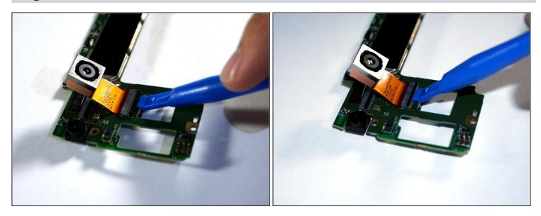
• Lift the locking bar on the ZIF connector that is under the rear facing camera with a plastic opening tool.
