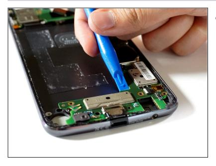
Place a plastic opening tool under the edge of the motherboard.
