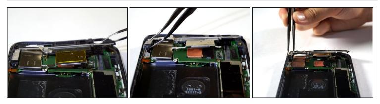
• Lift gently to completely remove speaker housing using tweezers.
