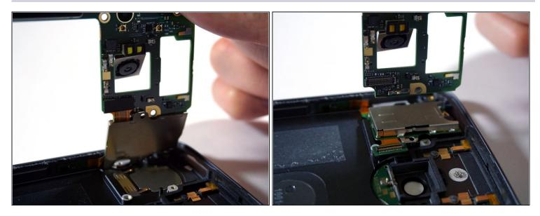
• Detach the connection on the bottom of the motherboard.
