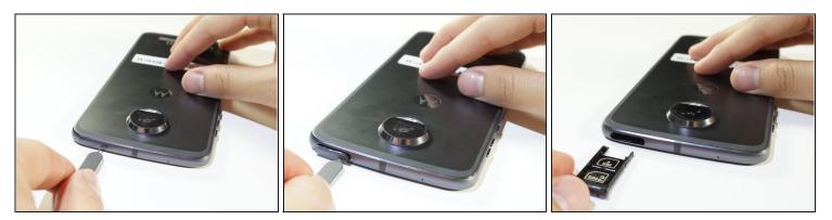
• Insert a SIM eject tool, bit, or a straightened paperclip into the hole in the SIM tray, located at the top left edge of the phone.
