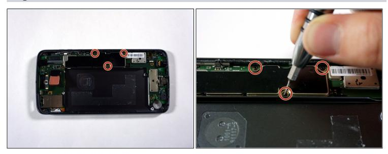
• Remove the three black 2.6 mm T3 Torx screws on the motherboard panel at the side of the phone with a screwdriver by turning counterclockwise.
