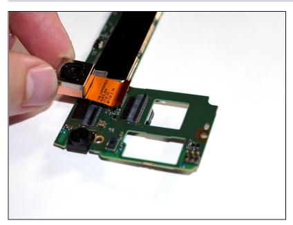
• Pull out the ribbon connector for the rear-facing camera.
