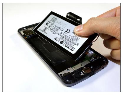
• Lift to remove the battery from the device completely.
