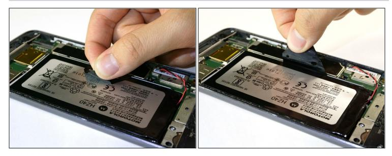
• Peel back the black tape that is located on the battery.
