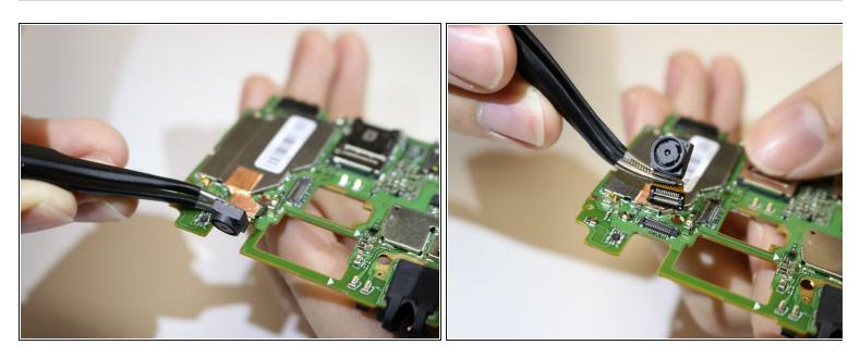
• Grab the connector with the tweezers and gently unplug the front camera from the motherboard.
