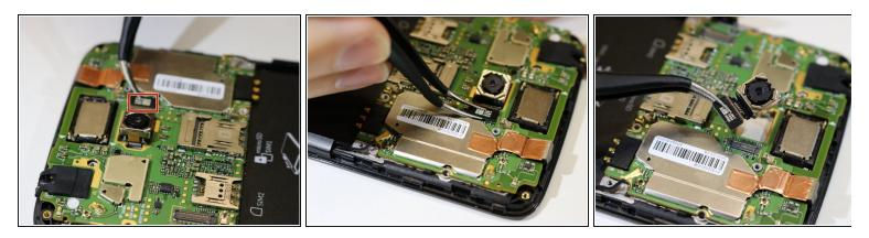
• Disconnect the marked connector with a pair of tweezers and remove the camera piece.
