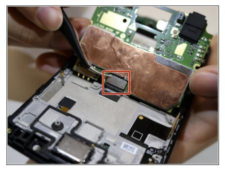
• Unplug the back connector from the motherboard using tweezers.
