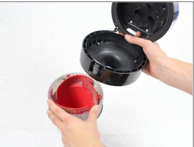
Unscrew the three 4 cm Phillips #3 screws located inside the dust filter compartment to detach the dust filter system.
