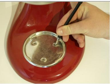
Using a #2 Phillips screwdriver, remove the three 13mm screws holding the bowl screw cap on by rotating them counterclockwise.
